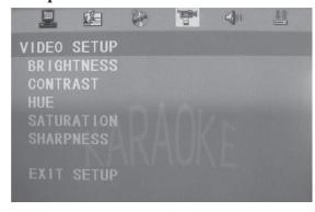
Unload the disc, press SETUP KEY to open the Setup MENU, then press Direction KEY [◀/▶] to select VIDEO SETUP (*see image above*). The SUB-MENU contains:
